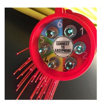
The Surface Cable of KONTINITRO SA works with the latest Optic Fiber Technology. It transmits the information through optical probes from the source to analyze to the Explomet 2 & Explomet-fo-2000 at 2/3 of the speed of light. It is specially designed for V.O.D measurements in all environment: quarry, mine, tunnel, underwater measurements, under vacuum measurements, laboratory & space program.
